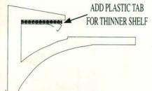
3) Install shelf. Check thickness of shelf. Your brackets are either for 3/8"~ 1/2" or 5/8"~ 3/4". They are pre set for the thicker capacity. If a thinner shelf is being used, peel mounting tape and carefully put plastic tab supplied in place (plastic side up - mounting tape down).
